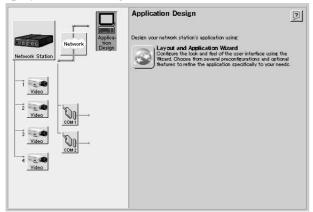
Clicking the (Layout and Application Wizard) icon displays the "Layout and Application Wizard". When the wizard is first run, a screen appears on which to select either [Layout] or [Application] settings. Select [Layout] to configure the monitor screen, or select [Application] to set alarm inputs and alarm event responses.
